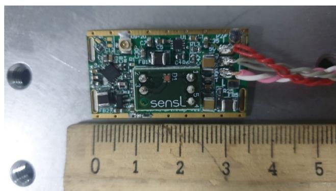
**Figure 1.** Picture of silicon photomultiplier (SiPM) on printed circuit board (PCB) board with amplifiers.
