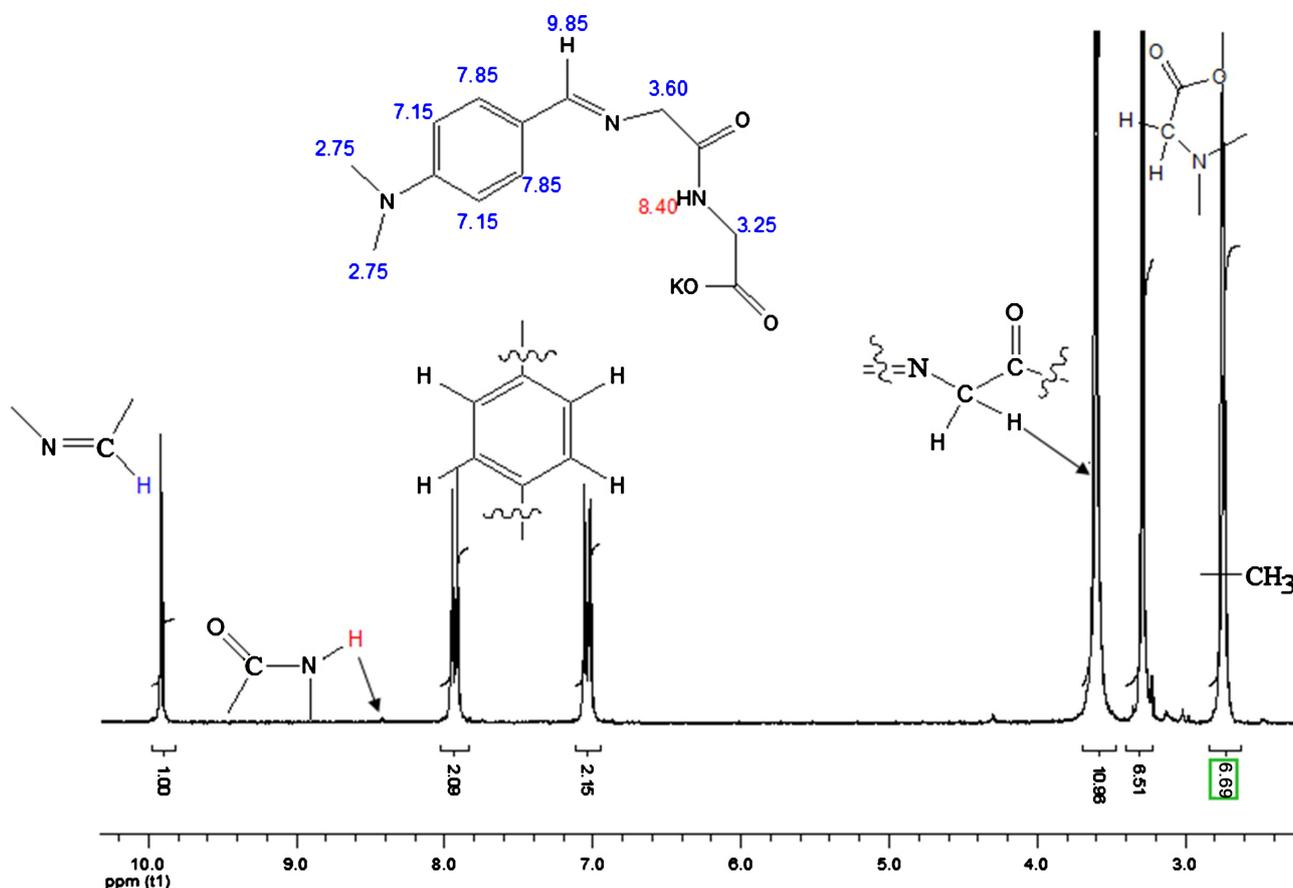
**Figure 2.** The  $^1\text{H}$ -NMR spectrum and proposed structure of glygly-DAB ligand (L).
