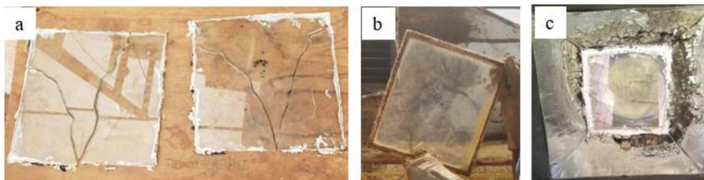
**Fig. 10. a) Broken ordinary panes (5 mm thick). b) Tempered panes of 3 mm thickness and 0.28 m side. c) Damaged secondary reflector made of self-adhesive mirror-effect film and wall-panes seal provided by silicone**
