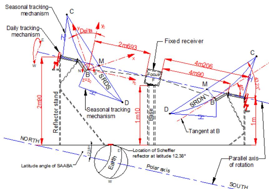
**Fig. 1. Configuration of the plastic waste (PW) melting unit with a pair of Scheffler reflectors facing each other. Scheffler reflector directed to the south (SRDS) and Scheffler reflector directed to the north (SRDN)**
