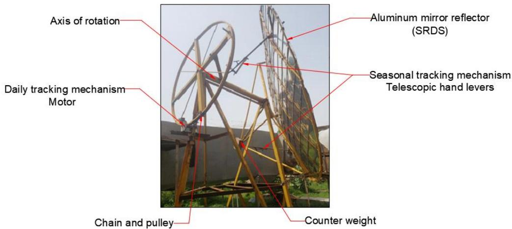
Fig. 7. Seasonal tracking mechanism using the telescopic levers of the SRDS. Saaba website
