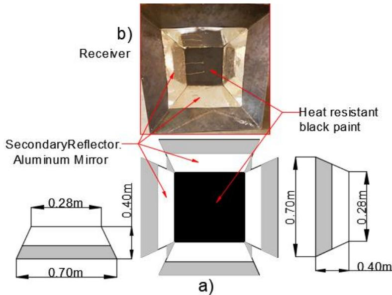
Fig. 2. a) Diagram of the secondary reflector. b) Photo of the secondary reflector
