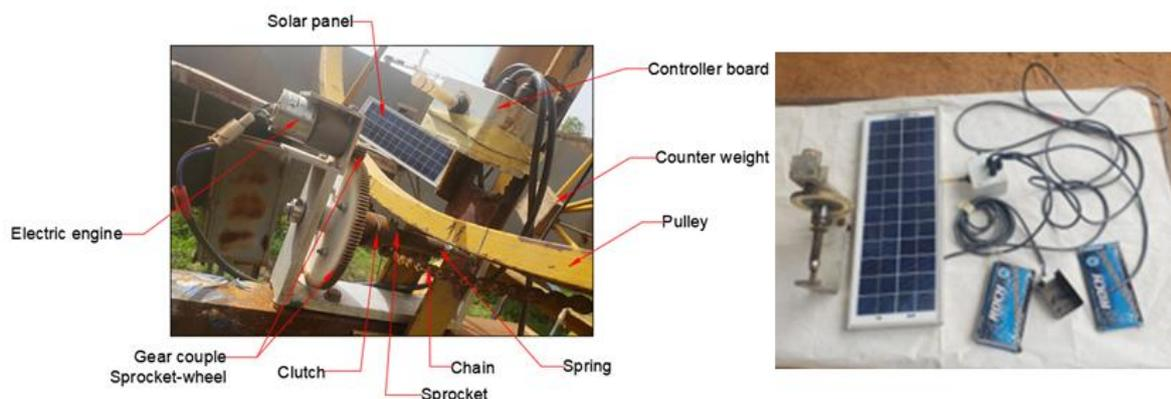
Fig. 6. a) Daily tracking mechanism mounted on the SRDS at Saaba (latitude 12.38°; longitude - 1.43°). b) Overview of the equipment used
