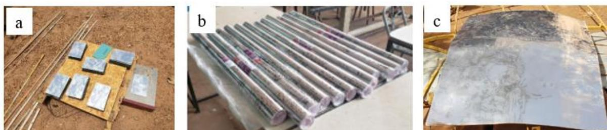
**Fig. 5. a) Pieces of glass mirror and Iron strips. b) Self-adhesive mirror-effect film. c) Aluminum Mirror**
