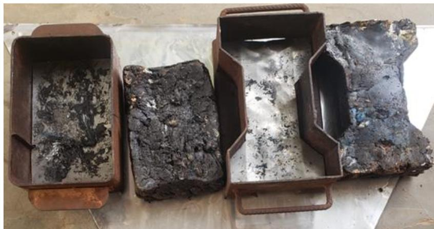
**Fig. 13. Pavers of the matrix of the composite material produced with molds of different shape on April 30, 2021**
