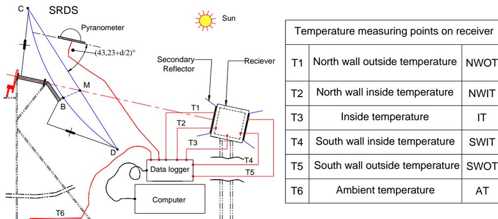
Fig. 8. Configuration diagram of the measurement equipment at Saaba.
