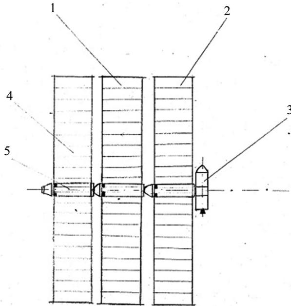
**Figure 7.** Structure of space train for the third cruise fulfillment.
