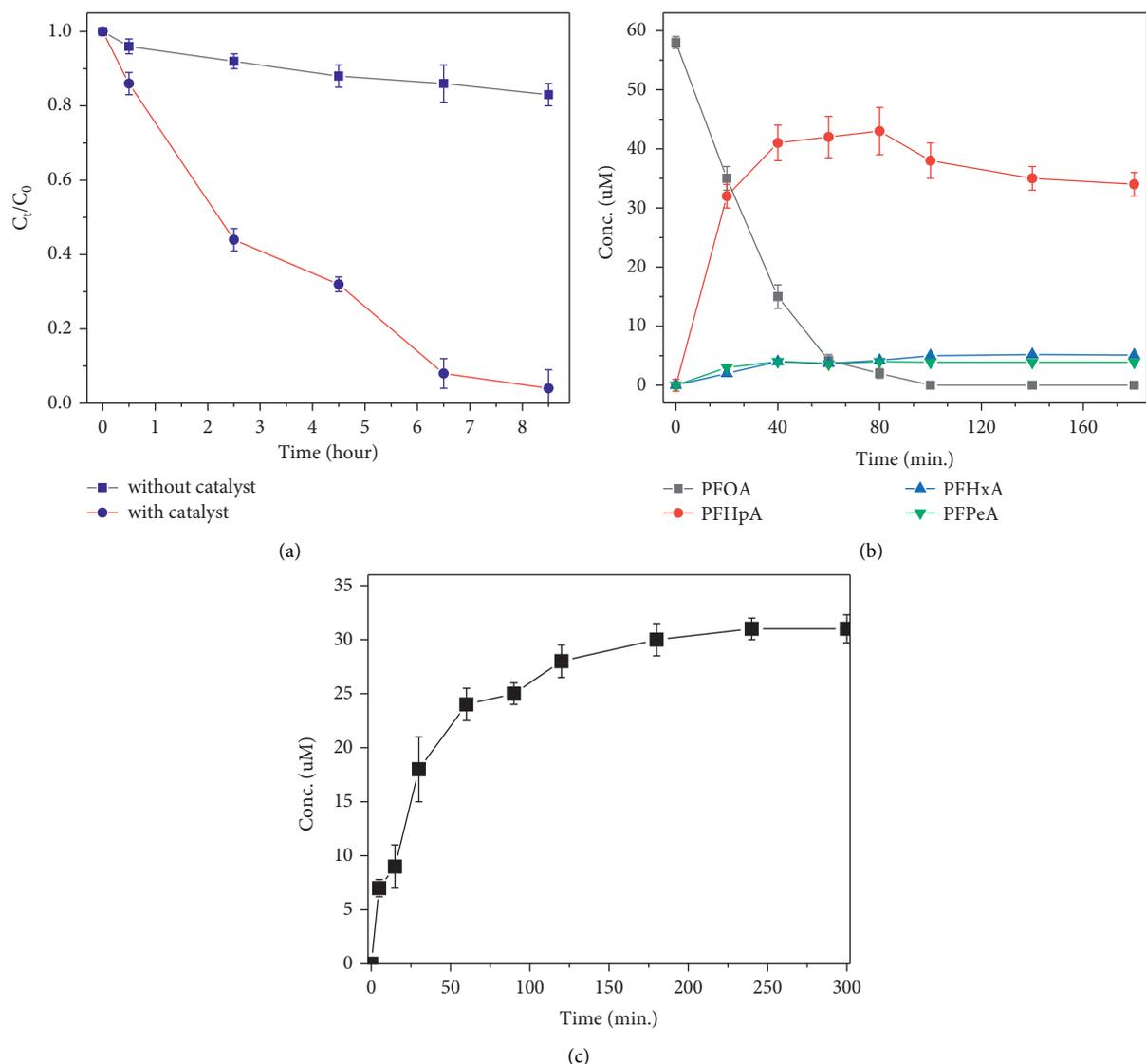
FIGURE 4: (a) PFOA photodegradation kinetic curves with and without  $\text{TiO}_2\text{-MWCNT}$  and (b) degradation and product curves of PFOA in the presence of  $\text{BiOI}_{0.8}\text{F}_2$  at pH 6.0 and  $25^\circ\text{C}$ . (c) Degradation and product curves of transformed PFOA from PFOSA in the presence of 0.2 M NaOH and 50 mM potassium persulfate.
